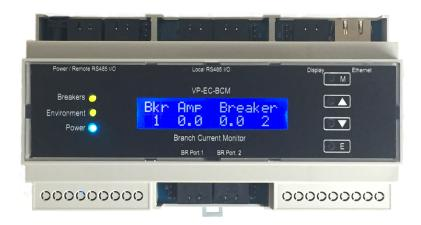
The VP-EC-DCIM-BCM-60 is a complete 60 breaker panel branch current monitoring system. Up to 2 VP-EC-BCM-42CT Interfaces can be connected for a total of 84 breakers. Each interface transmits its current readings to the gateway via Modbus RTU RS485 protocol. The VP-EC-BCM-Gateway's built in web server allows the user to program all alarm and operating settings for the breaker variables. Email alerts are programmed for Warning, High, and Zero Load Alarm.
