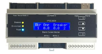
The VP-EC-DCIM-BCM-84 is a complete 84 breaker panel branch current monitoring system. Up to 2 VP-EC-BCM-42CT Interfaces can be connected for a total of 84 breakers. Each interface transmits its current readings to the gateway via Modbus RTU RS485 protocol. The VP-EC-BCM-Gateway's built in web server allows the user to program all alarm and operating settings for the breaker variables. Email alerts are programmed for Warning, High, and Zero Load Alarm.
