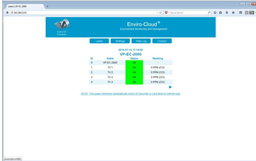
The second display mode is the extended, or long, display which adds the Temperature, Relative Humidity, Battery, Last Update, Pulse, and Signal (Strength) columns to the compact display. Toggle between these display modes using the ▶ and ◀ symbols at the bottom, right corner of the table.
