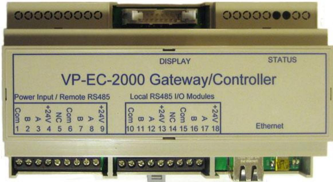
The VP-EC-2000 Gateway/Controller is the heart of the system. This unit contains the main processor and firmware, Ethernet port and RS485 Ports. The optional Zigbee Coordinator module is also contained in this module.
