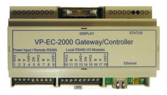
The VP-EC-2000 Gateway/Controller is the heart of the system. This unit contains the main processor and firmware, Ethernet port and RS485 Ports. The optional Zigbee Coordinator module is also contained in this module.
