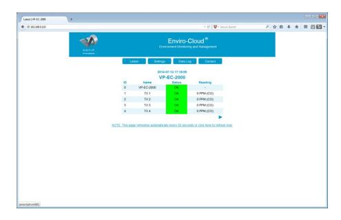
The second display mode is the extended, or long, display which adds the Temperature , Relative Humidity, Battery, Last Update, Pulse, and Signal (Stregnth) columns to the compact display. Toggle between these display modes using the > and < symbols at the bottom, right corner of the table.
