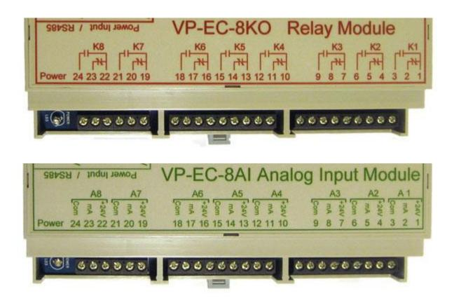
For remote RS485 Devices, the wiring +24VDC, DATA A, DATA B, and COMMON are connected to the LOCAL RS485 Port Clearly identified on the VP-EC-2000 Gateway / Controller DIN Moule.
